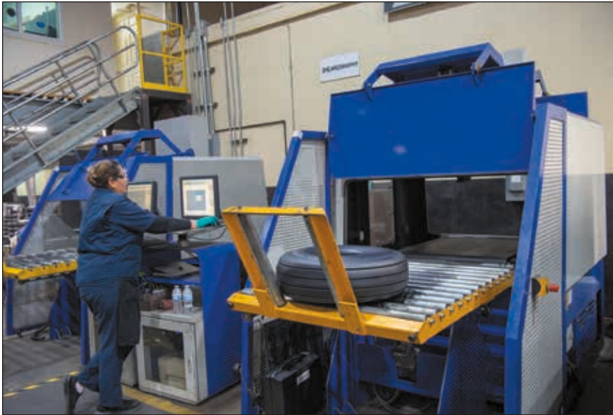
That's a retread in the Shearography Measuring System machine in the top photo, and a check of new rubber depth gauge in the middle. The tire at the bottom is ultimately rejected during the weathering check portion of inspection.
