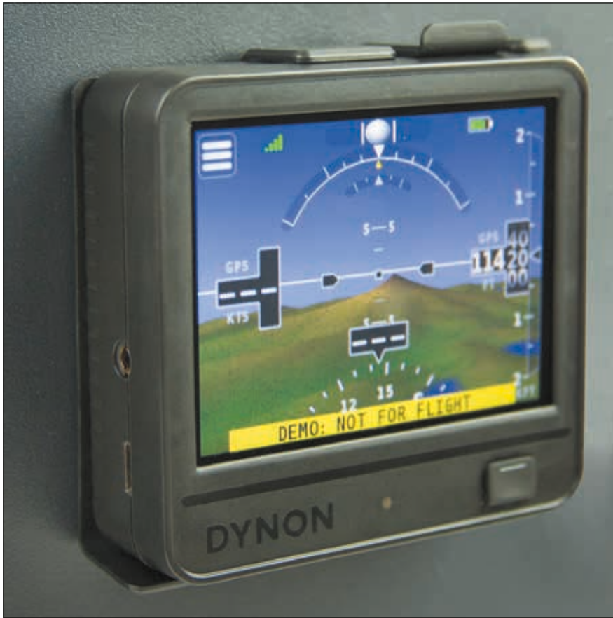
That's the D3 in the pinch panel mount in the main image to the left. It's secure and easy to remove and reinstall. The bottom image is the D3 secured to a RAM window suction mount. The big display in the photo is Dynon's SkyView Touch PFD.
