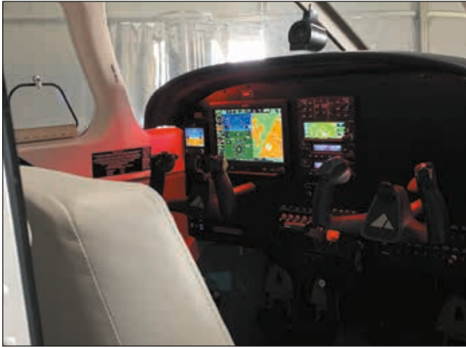
The Pilot 100i model comes with Garmin's G3X Touch integrated avionics and a center stack suited for instrument flying. It includes the GFC500 autopilot, G5 EFIS backup and Garmin's newly introduced GNX375 WAAS IFR navigator with ADS-B In and Out.
