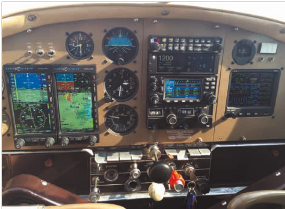
William Solaga's reworked 195 panel has a pair of Aspen flight displays, an ADS-B transponder and a big-screen engine display for minding the radial engine, top. The 195 panel in the middle is more old school. The throttle and prop controls are placed in the subpanel, bottom.
