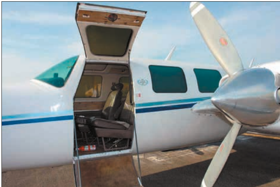
Pilot and passengers ingress and egress the cabin of an Aerostar via a clamshell door on the left side of the fuselage.
