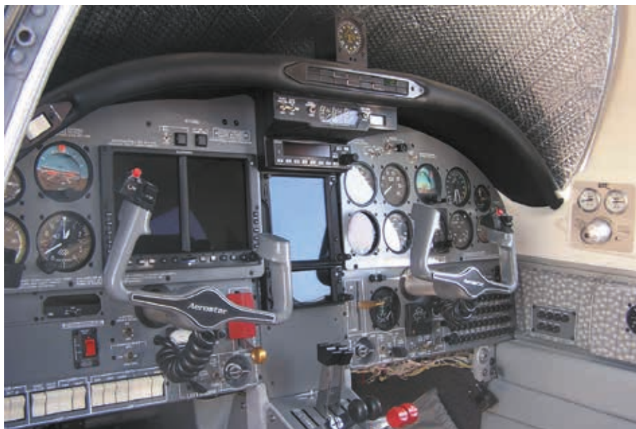
When searching the used Aerostar market, buyers will find a wide variety of avionics configurations. The panel in the top image has round-gauge flight instruments and the one at the bottom has Garmin glass.
