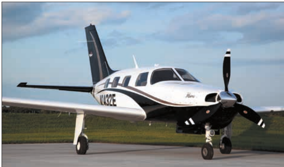
The Matrix, above, is lighter and less complex than a Malibu/Mirage without its pressurization system.
