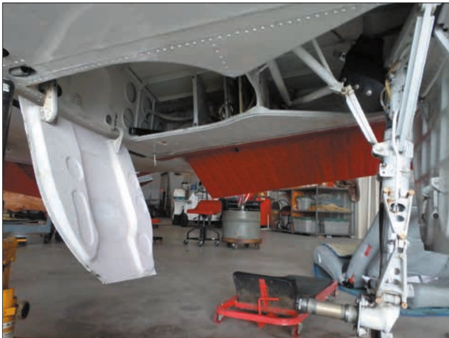
No matter the vintage, a close look at the landing gear during a pre-purchase inspection is a must. Corrosion and rigging issues aren't uncommon.
