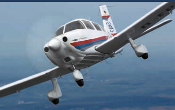
The Archer DX pictured above has Continental's CD-155 diesel engine and a $400,000 price tag.
