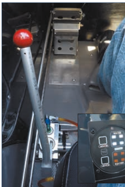
The Aerocets have manually operated hydraulic gear, above, with an electronic nanny to remind of gear position prior to touchdown.
