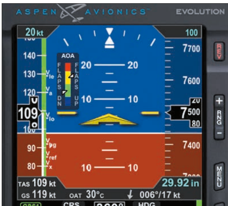
AoA indications are logically displayed to the right of the airspeed tape on the Evolution PFD, left photo, and on a dedicated page within the Evolution MFD, right photo.
