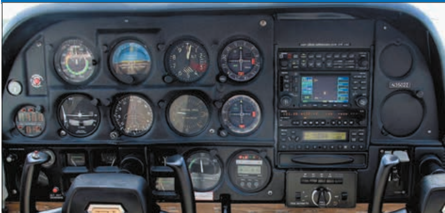
Used avionics and steam gauges like the ones in this Cessna Cardinal panel, left, might be a good option for a budget upgrade. Still, the Garmin GMA340 audio panel, GNS430W, SL30 navcomm and GTX330ES ADS-B in that stack could run close to $20,000.
