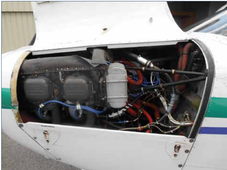
Upper cowling halves open wide, providing excellent, rapid access to engine and accessories.
