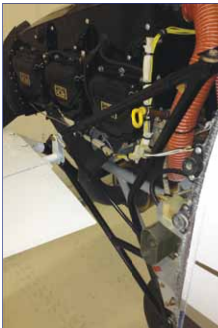
Push-rod-operated canard mounts outside the engine mount, above; brake line is routed behind main gear leg to avoid snags, above right, and gear leg has stainless steel leading edge.
