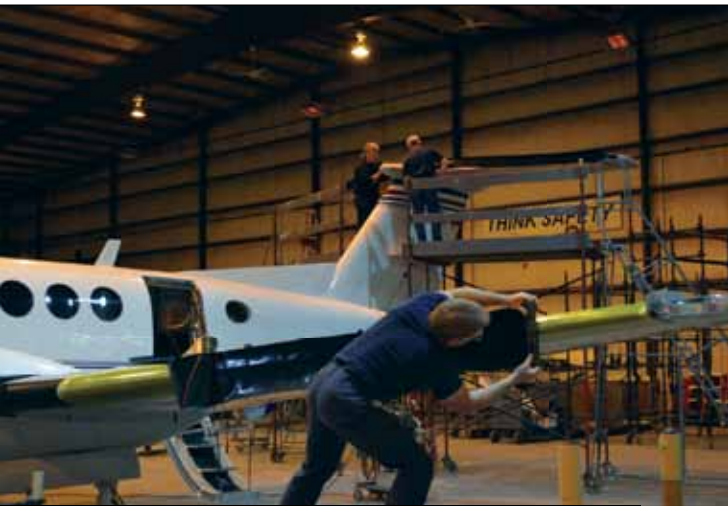
Preparing for boot installation means cleaning the area down to bare aluminum, top. Installing a FASTboot on a King Air at the Goodrich Service Center.
