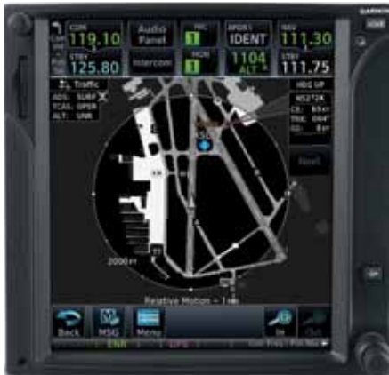
A Garmin SafeTaxi diagram showing ADS-B-equipped aircraft and vehicles on the ground as displayed on a GTN 750.
