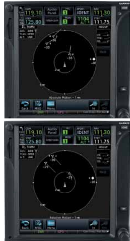
Traffic information received by the GDL 88 as displayed conventionally on a GTN 750, top. Using TargetTrend, the movement of other aircraft relative to yours is displayed, above, allowing faster threat assessment.
