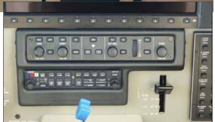
Garmin's G1000, top photo, is standard equipment in the Matrix/Mirage. So is a GFC700 autopilot, right, whose control panel lives under the MFD. G1000 keyboard is on the lower shelf of the power pedestal, bottom photo.
