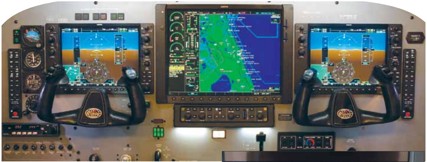
Garmin's G1000, top photo, is standard equipment in the Matrix/Mirage. So is a GFC700 autopilot, right, whose control panel lives under the MFD. G1000 keyboard is on the lower shelf of the power pedestal, bottom photo.
