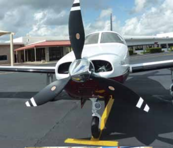
The Matrix's TIO-540-AE2A swings a three-blade scimitar prop, left. Like most manufacturers, Piper has converted exterior lighting to low-draw LEDs, lower photo.
