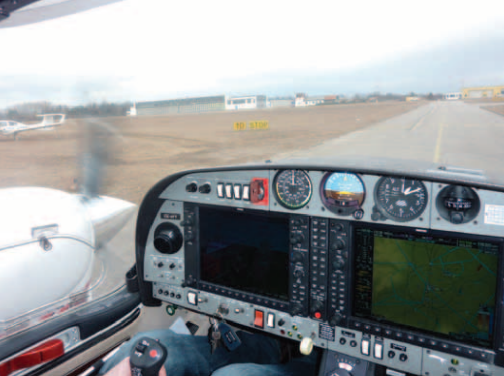
DA42 V1s will have the Garmin G1000, top. Diamond retained the automated ECU test function, left. Power control is single lever.
