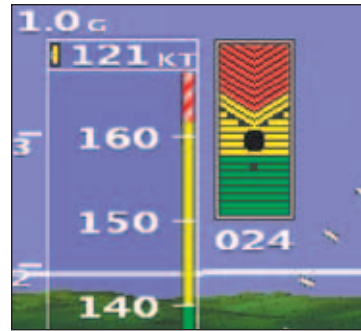
Advanced Flight Systems derives AoA from ports drilled in the top and bottom of the wing. Their Pro and EFIS system display AoA numerically and with color-coded bars. There's also a simple, eight-LED option.
