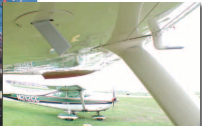
The Alpha Systems probe mounts in an inspection cover at least two feet outboard of the prop (below). Another display option is the original, a.k.a. legacy, display (left).
