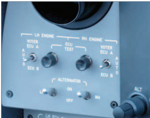
DA42 V1s will have the Garmin G1000, top. Diamond retained the automated ECU test function, left. Power control is single lever.
