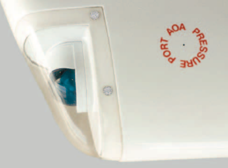
Advanced Flight Systems derives AoA from ports drilled in the top and bottom of the wing. Their Pro and EFIS system display AoA numerically and with color-coded bars. There's also a simple, eight-LED option.
