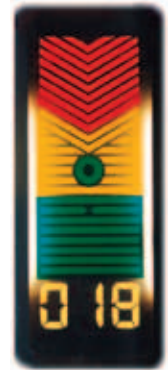
Advanced Flight Systems derives AoA from ports drilled in the top and bottom of the wing. Their Pro and EFIS system display AoA numerically and with color-coded bars. There's also a simple, eight-LED option.
