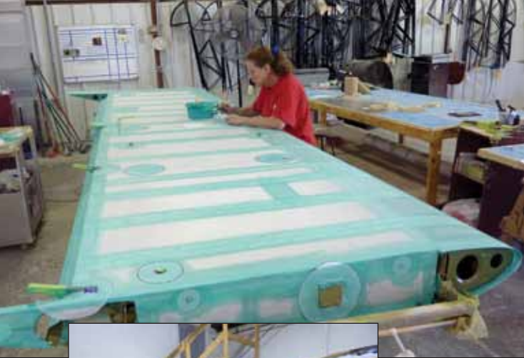
Wings are covered with modern Poly-Fiber, left. Fabric is riveted to ribs. The fuselages still contain wood, used for stringers and bulkheads to hold the fabric shape.
